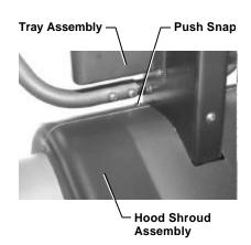
NOTE: TO REPLACE PUSH SNAP, POSITION INNER PIN SO THE HEAD OF THE PIN IS OUT AT THE TOP.
